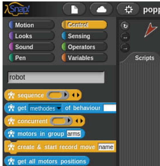
Figure 10. An example of code for the programming of Ergo Jr robot using a visual programming system Snap!
